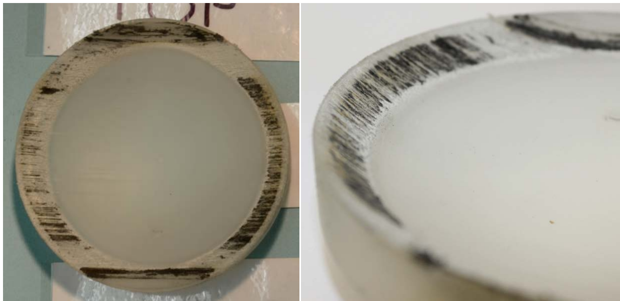
Fig. 7. Kynar® blind seat for three-way, PBM, 3-inch slurry valve (TV8) after being rinsed. Image on right is a close-up of left side of the blind seat.
