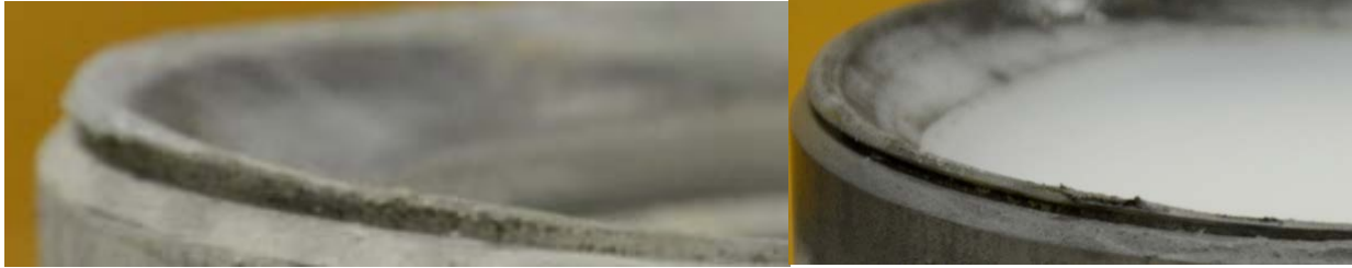
Fig. 8. Left: Tefzel® seat of three-way, PBM, 3-inch slurry valve (TV1) still in retaining channel of flush port flange stem. Right: Tefzel® blind seat still in retaining channel of flange stem from three-way, PBM, 3-inch drain valve (TV3). Note: Original installation of both pictured seats had the top of each seat flush with the top of the retaining channel.
